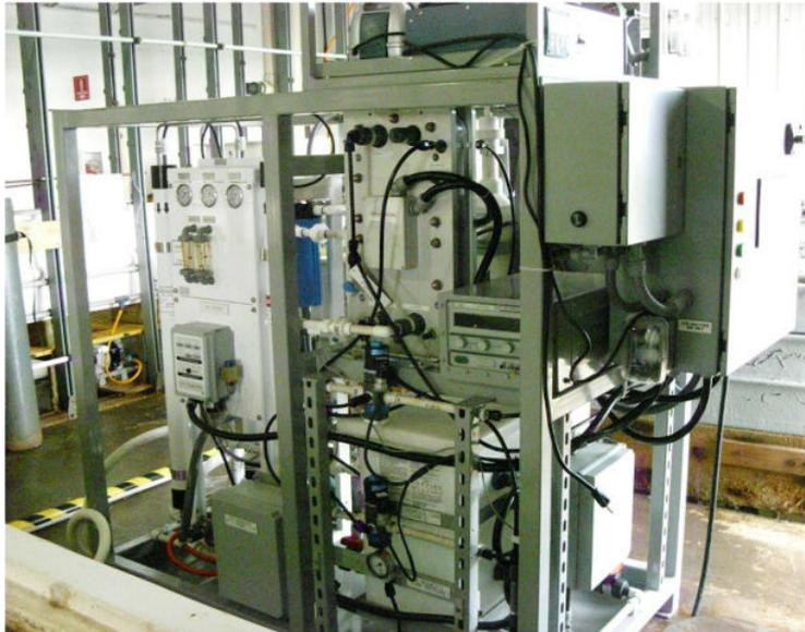
*Electrochemical Acidification Carbon Capture Skid. The acidification cell was mounted onto a portable skid along with a reverse osmosis unit, power supply, pump, carbon dioxide recovery system, and hydrogen stripper to form a carbon capture system.*
