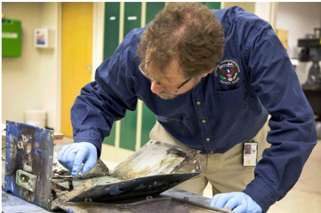
***NTSB Materials Engineer Matt Fox examines the casing from the battery involved in the JAL Boeing 787 fire incident in Boston.***
