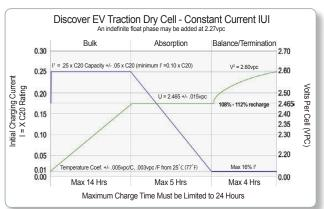
■ NOTE: This algorithm uses a pulse termination criterion. As a safety precaution during the Finish phase, if the average cell voltage, or volts per cell (ypc), exceeds V2 and the charger output has been on for more than 30 seconds, the output is shut off until the vpc falls to V3. The finish phase then resumes and this "pulsing" continues until the target overcharge (108% - 112%) is reached.
